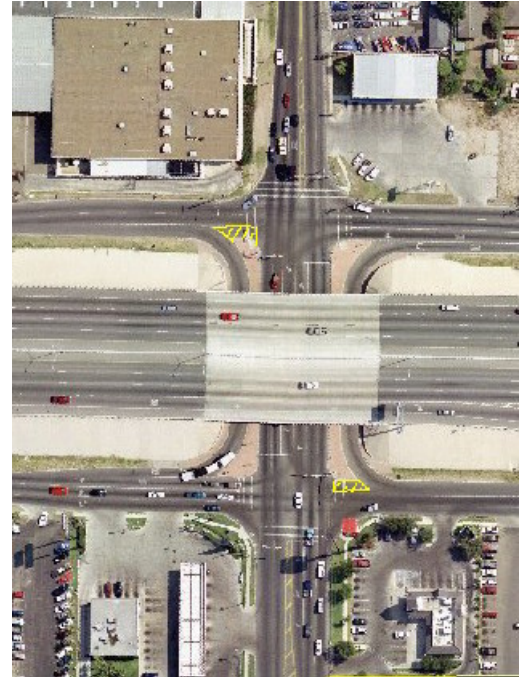
Figure 4.3-4 Cross Hatch Added
